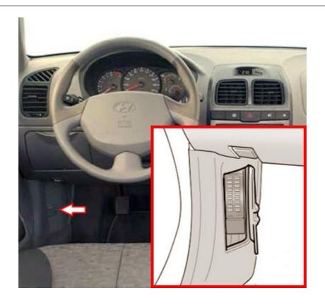
Located on the left pillar under the dashboard, behind the protective cover.
