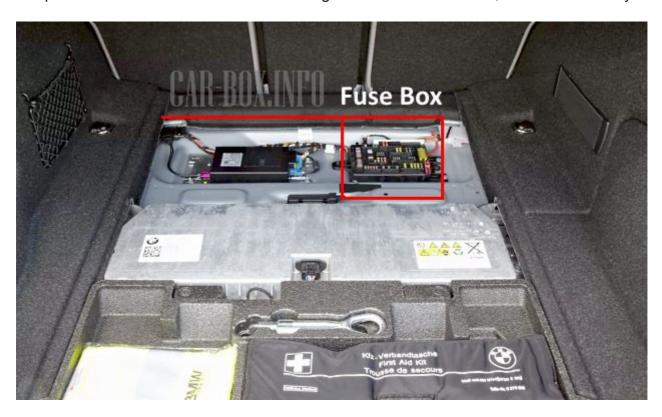
The main fuse box is in the center behind the floor pan.
