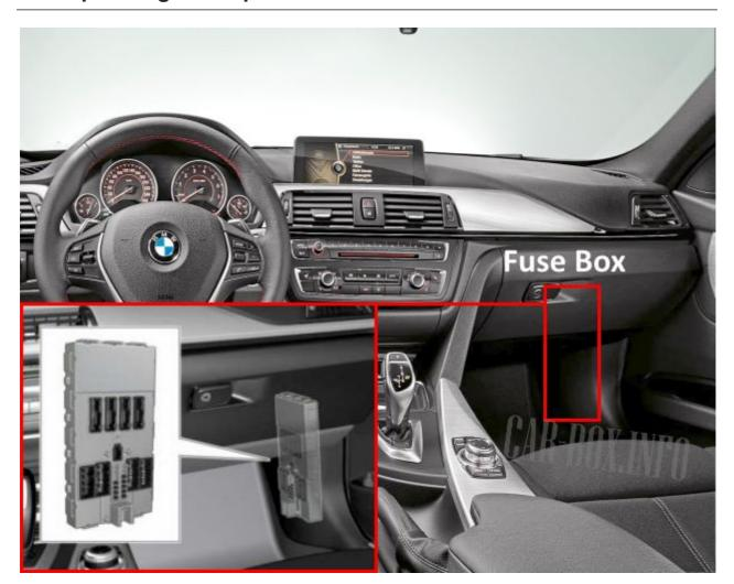
The unit is located on the passenger side on the front pillar.
