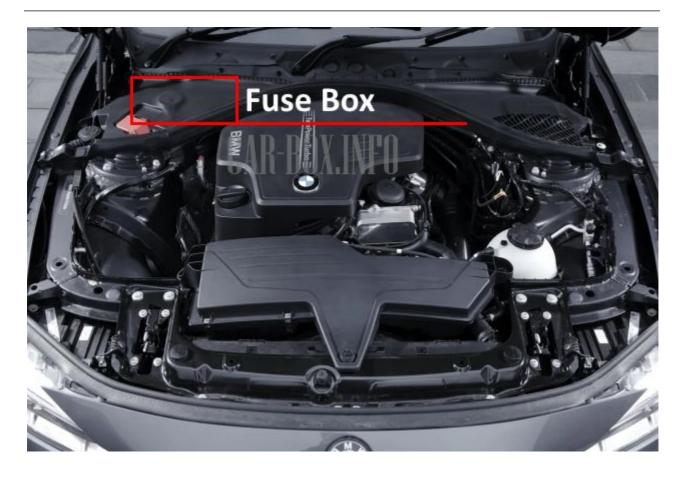
The main unit is located on the right side, closer to the windshield. To access it, you need to unscrew the mounting screws of the protective cladding. Next to it there are some relay modules and power fuses.
