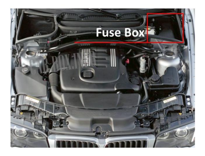
The unit is located on the left side of the engine compartment, behind the plastic cover.
