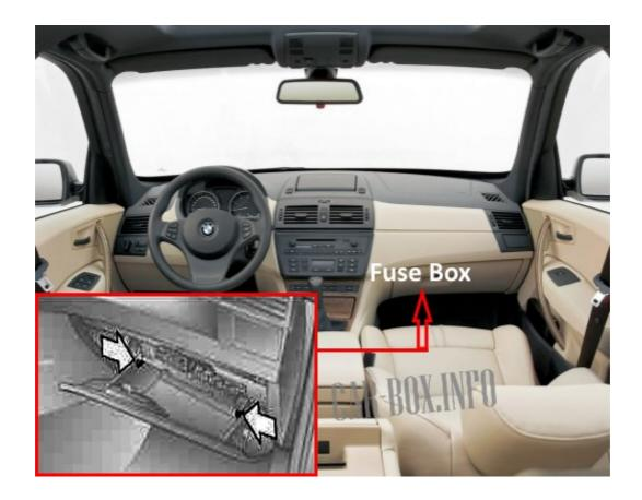
The mounting block is located behind the glove compartment. In order to access it, unscrew the two clips and pull it downwards.
