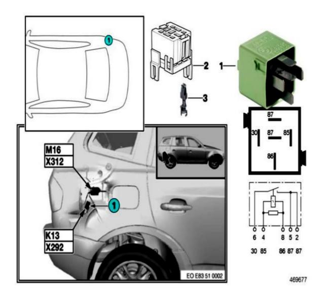
The rear window heater relay module is located under the right side trim.
