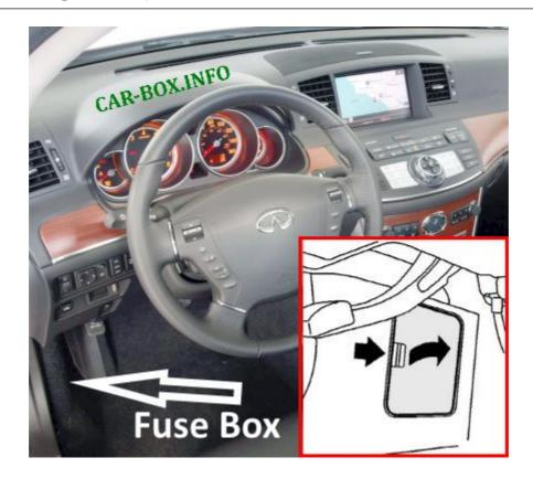
There is one fuse block with fuses in the passenger compartment; some relay modules are located on its back side.
