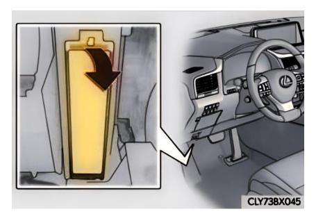
The fuse box is located under the dashboard on the driver's side.
