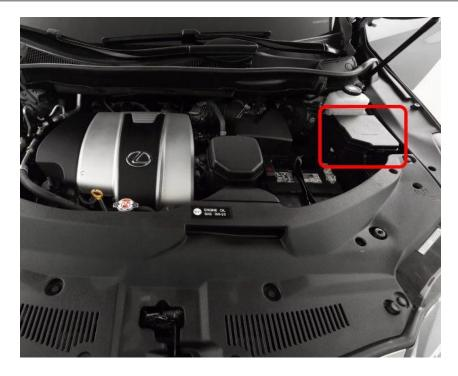
The fuse box is located on the left side of the underhood.
